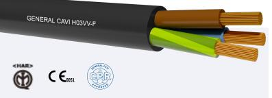
Class 5 flexible copper conductor. PVC Insulation in TI2 quality. PVC sheath in TM2 quality.
